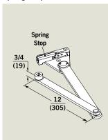
Heavy-duty parallel arm with spring assisted dead stop function. Available in non-hold open and thumb turn hold open. Units can be installed to achieve either stop or stop and hold open at 85°, 90°, 100°, and 110°. Maximum opening is 110° (conditions permitting). Arm is non-handed. Non-hold open arm illustrated.
