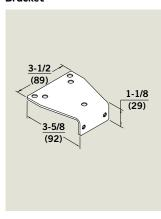
P89 — Furnished standard with 8900 P Series closer non-hold open and plunger hold open parallel arm applications. Spacer block furnished standard for use with narrow stop applications.
