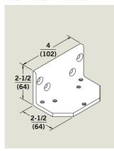
**FTHD** — For use with all 8900 Series DS and SPA applications where flush transom conditions prohibit normal installation of soffit bracket.
