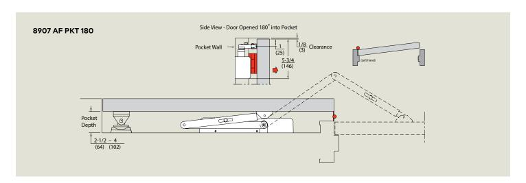
The recommended method for hanging the door is via the use of butt hinges, which create optimum unobstructed space when the door is in the pocket. Alternate methods using 3/4" Offset Pivots, Swing Clear Hinges, or Continuous Hinges are available. When using alternate methods, note where the pivot point of the hinge or pivot locates the door's angle of opening in order to determine the pocket depth.
