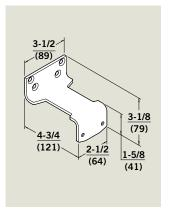
PFT — For all 8900 Series closer hold open and nonhold open parallel arm installations where flush transom conditions prohibit use of P89 or PHB bracket.
