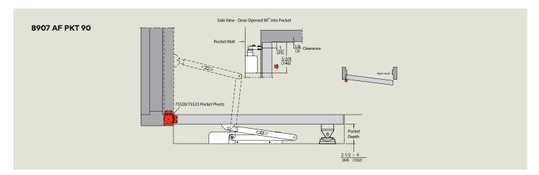
All dormakaba pocket door closers, combined with a dormakaba EM Series wall magnet, create a held open flush door until power is interrupted or the door is manually shut. See EM and LM Series product brochures for specific magnet and pivot information.
