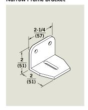
**NFHD** — For use with all 8900 Series DS and SPA applications where total frame depth is less than 4-1/2" (114 mm), prohibiting use of standard spacer block. NFHD bracket is used in lieu of block supplied with arm.
