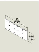
**DP89** — For parallel arm installation of 8900 Series closers when top door rail is less than 5-3/4" (146 mm) for non-hold open and plunger hold open. When top door rail is less than 6" (152 mm) for friction applications (assuming 5/8" (16 mm) stop dimension).
