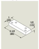
**BS** — For use with all 8900 Series P89, PD, and PHB applications installed on cased frames with applied blade stops. This block is used in conjunction with the spacer furnished with the arm to provide adequate clearance for the blade stop.
