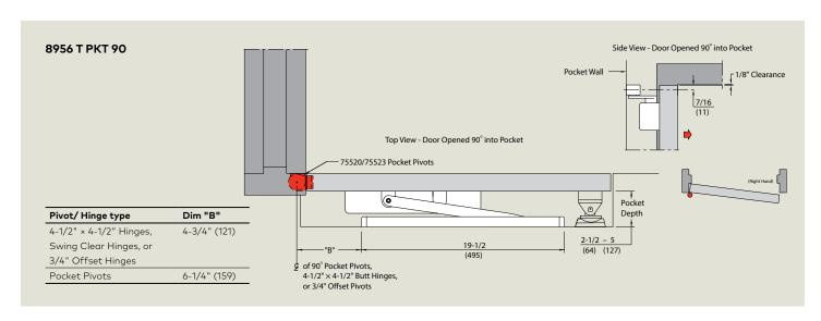
All dormakaba pocket door closers, combined with a dormakaba EM Series wall magnet, create a held open flush door until power is interrupted or the door is manually shut. See individual EM and LM Series product brochures for specific magnet and pivot information.
