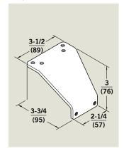
PD — For 8900 Series closer non-hold open parallel arm applications to clear a surface-applied stop/holder.
