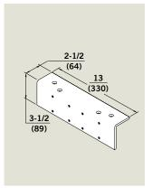
AB89 - For installation of 8900 Series closers where parallel arm and top jamb applications are not practical due to low overhead ceiling clearance, narrow frame face, or unusual trim conditions. This bracket can also be used to provide clearance for a surfaceapplied stop/holder.
